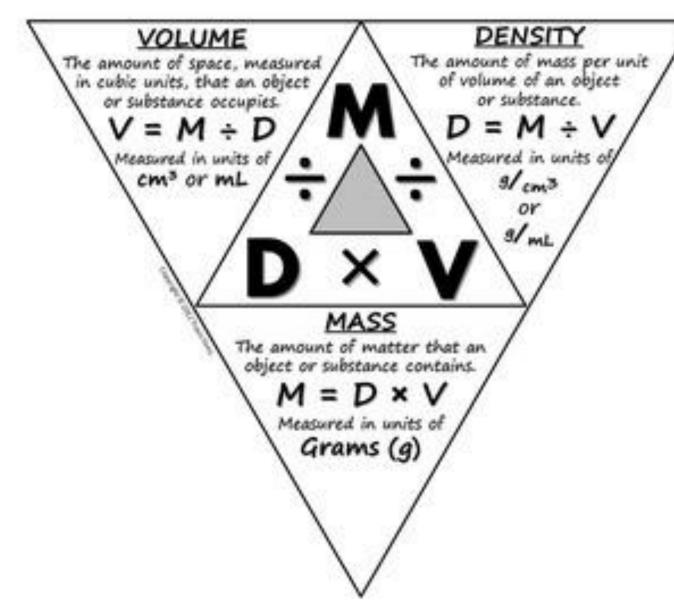
The formula for density can be rearranged to solve for for the required unit.
